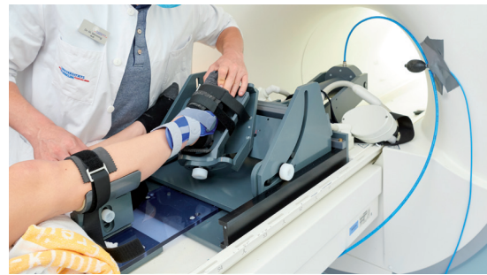
Fig. 1: 3SAM study design (3D arthrometric ankle measurement using MRI); Image: Udo Schönewald
